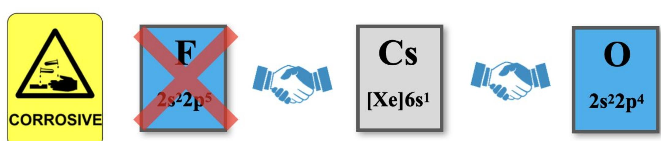
Fluorine is corrosive to diamond anvil cells, making the experimental verification of the above predictions extremely challenging.
